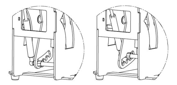
Moving the contact point of the springs to the front lowers the closing force, while moving to the rear increases it. Please note that sufficient force is required to ensure automatic opening of the press - the opening force decreases or increases along with the closing force.
