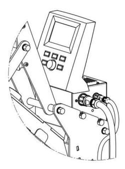
Plug the supplied C13 cold device cable into the back of the controller box and connect it to a safety socket, which must be equipped with a grounded connection, protection via fuse and ground fault circuit interrupter.
