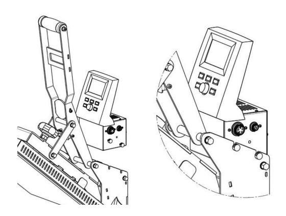
Attach the small 6-pin plug from the rear side of the heat press base to the appropriate socket on the outer right side of the controller box.
